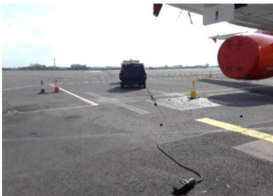
Trailing cable pulled from the aircraft
