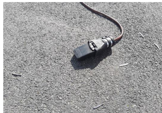
Damaged GPU plug
